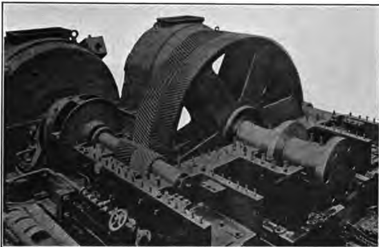
FIG. 137.— Wulsty Castle : Reduction Gearing with Cover Removed
